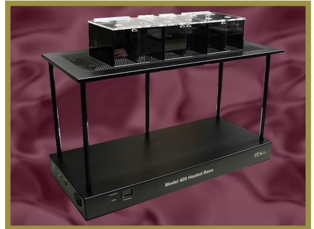
Mesh is interchangeable with glass in any one of the IITC plantar and or combination plantar/tail flick systems. A cost saving feature that allows users to use one stand for two separate tests.
